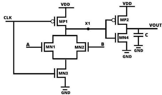
Fig. 2. CMOS based Domino OR gate
