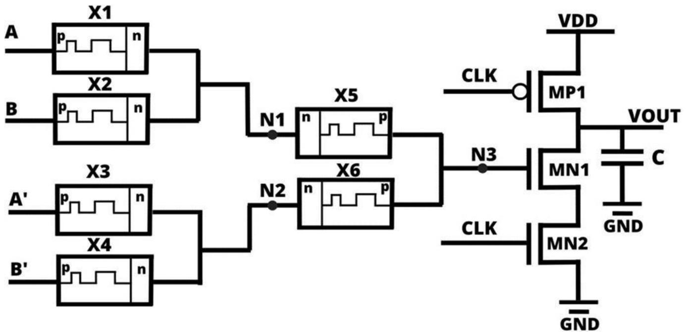
Fig. 7. Proposed Memristor-based Dynamic Exclusive-OR gate
