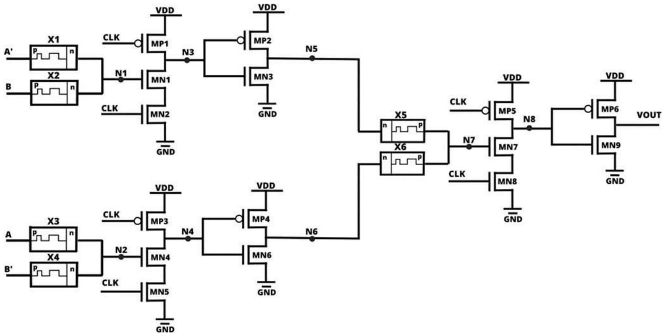
Fig. 6. Existing memristor-based dynamic Exclusive-OR gate
