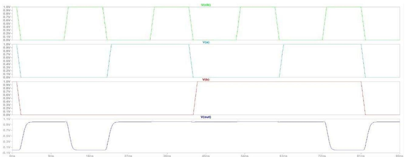
Fig. 8. Timing waveforms for Proposed Memristor-based Dynamic Exclusive-OR gate
