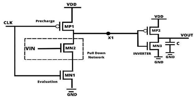
Fig. 1. CMOS Based Domino Buffer
