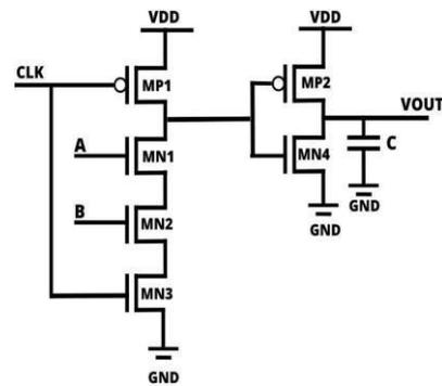
Fig. 3. CMOS based Domino AND gate
