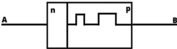
Fig. 5. Schematic symbol of memristor
