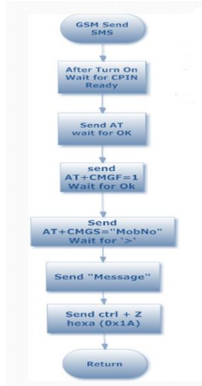
Figure 3. Flow chart to send a message using the GSM modem
