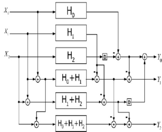
Figure 3: FFA Based FIR Filter for L=3
