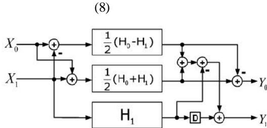
Figure 4: Proposed FIR filter for two-parallel implementation
