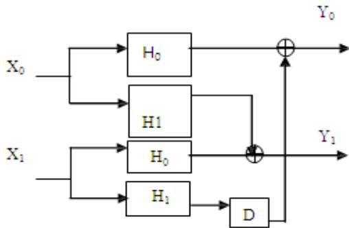
Figure 1: Traditional parallel FIR filter for L=2
