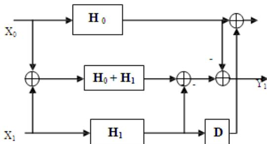
Figure 2: FFA Based FIR Filter for L=2
