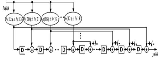
Figure 5: Subfilter block implementation with symmetric coefficients
