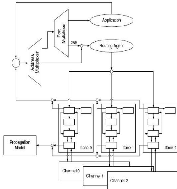
**Figure 2: Mobile Node Architecture with Multi-channel support**
