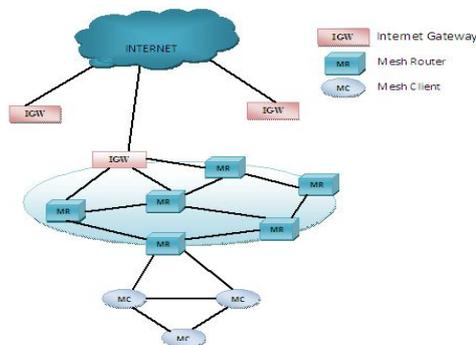
Figure 1: The network structure of a typical WMN
