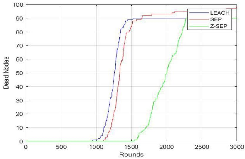
Fig 4: Number of Dead Nodes in LEACH vs SEP vs Z-SEP
