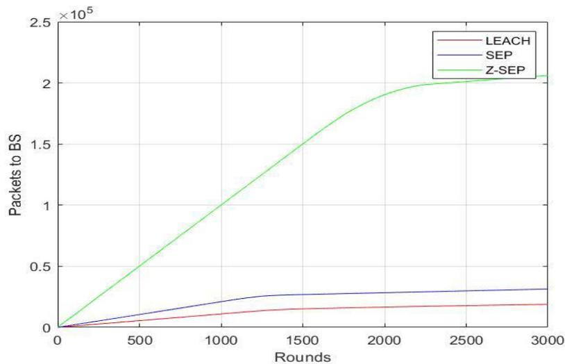
Fig 6: Number of packets to BS in LEACH vs SEP vs Z-SEP
