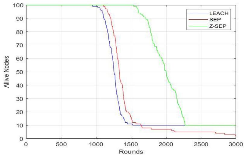
Fig 5: Number of Alive Nodes in LEACH vs SEP vs Z-SEP
