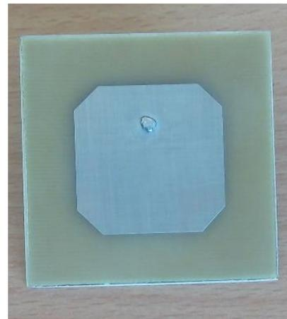
Fig.1.7 Fabricated Antenna
