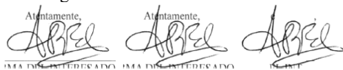
Fig. 7. Binarized signed area of a check I_D(x,y) (left), result of line removing procedure (middle), after reducing the amount of residual text I_{GD2}(x,y) (right).
