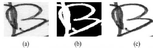
Fig. 5. Segmentation procedure. Details of (a) original image I(x, y) with 256 gray levels, (b) binarized and noise reduced signature I_{NR}(x, y) , (c) segmented signature I_G(x, y) with white background.
