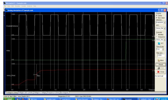
Fig: 4.2 Characteristic waveform for Conventional 6T SRAM
