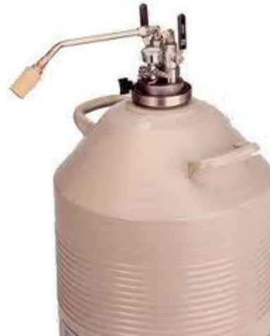
Figure 2 Dewar for storing liquid nitrogen
