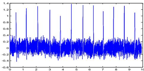
Figure 2: Noisy ECG signal (contain 50 Hz power line noise and motion artifact noise)
