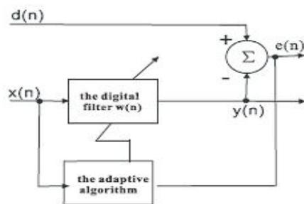
Figure 4: general Adaptive filtering diagram
