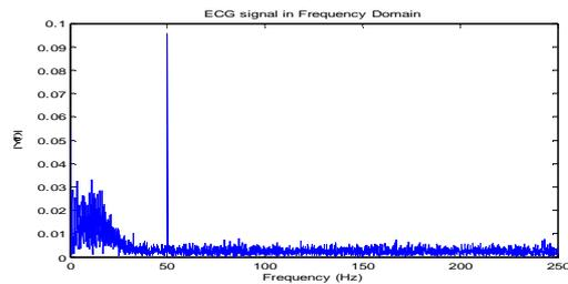
Figure 3: Noisy ECG signal (contain 50 Hz PLI and motion artifact noise) in frequency domain
