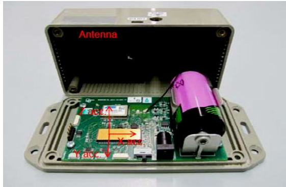
Fig8: Packaged accelerometer module with axes
