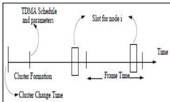
Fig 8. Time line for APTEEN
