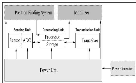
Fig 1. The components of a sensor node
