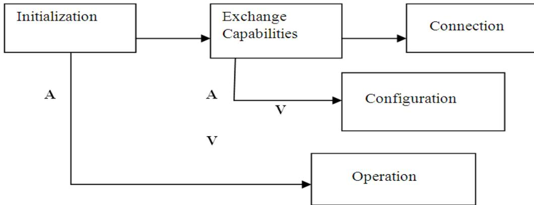
Fig.2 State machine for Wireless network control protocol
