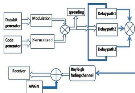
Figure 1: Block diagram of generic SSM transmitter.
