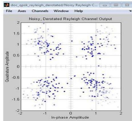
Figure 4: Scatter plot output after AWGN noise.
