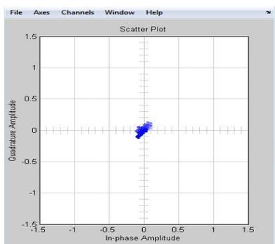
Figure 10: Scatter plot output after MLSE equalization.
