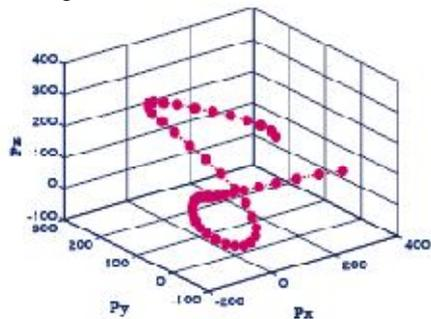
Fig. 8 : Variation of End-Effector Position Vector when all Joint Angles are varied uniformly and simultaneously.
