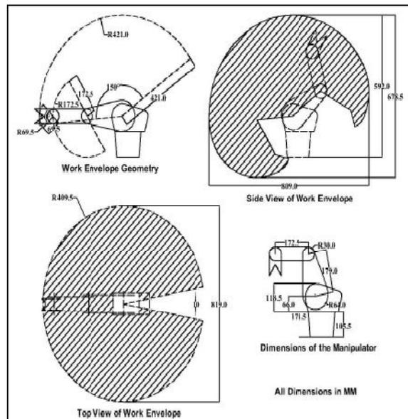
Fig.3 : Manipulator Design Specification
