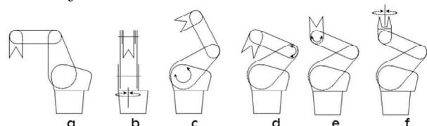
Fig. 4 : Various Motions of the Manipulator Parts 5
