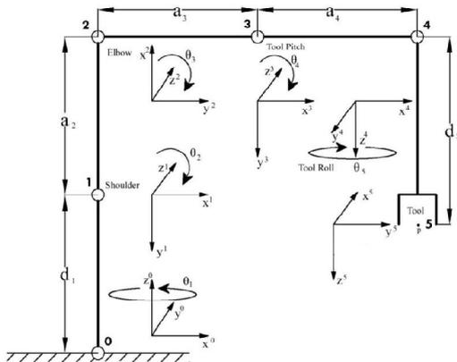
Fig. 5 : Link Coordinate Frame of the Manipulator
