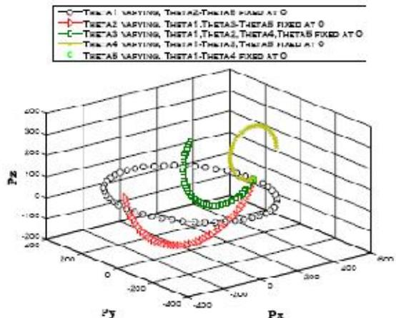
Fig.7: Variation of End-Effector Position Vector when one Joint Angle is varied while others are Zero.
