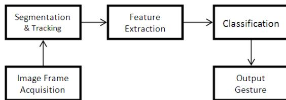
Figure 1: Block diagram for gesture recognition system
