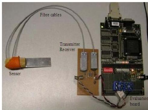
Figure 9. Assembly of opto-tactile sensor
