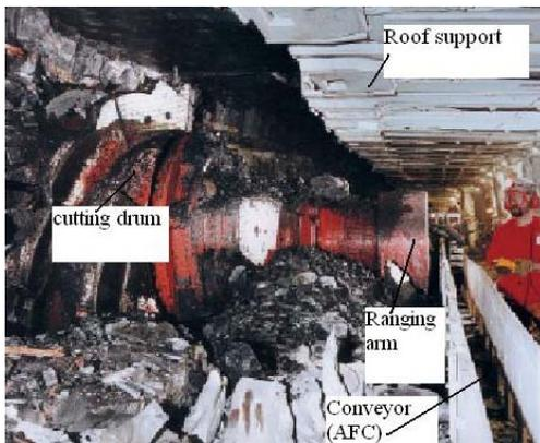
Figure 1. Shearer machine model EL 1000/3000 (courtesy DBT).
