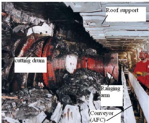
Figure 1. Shearer machine model EL 1000/3000 (courtesy DBT).
