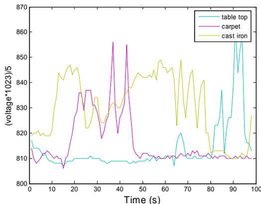
Figure 10. Surface texture evaluation by opto-tactile sensor
