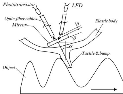
Figure 8. Opto-tactile sensor for object surface recognition.
