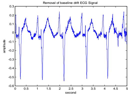
Figure 6. ECG signal after removal of baseline drift
