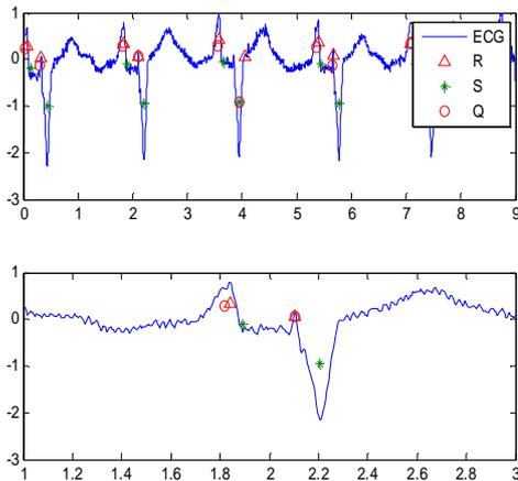
Figure 5. ECG signal after applying Pan Tompkins algorithm
