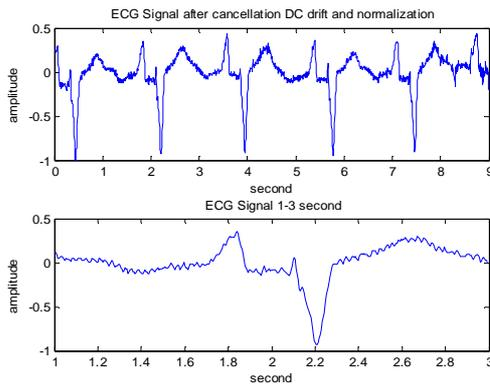
Figure 4. ECG signal after cancellation of DC drift
