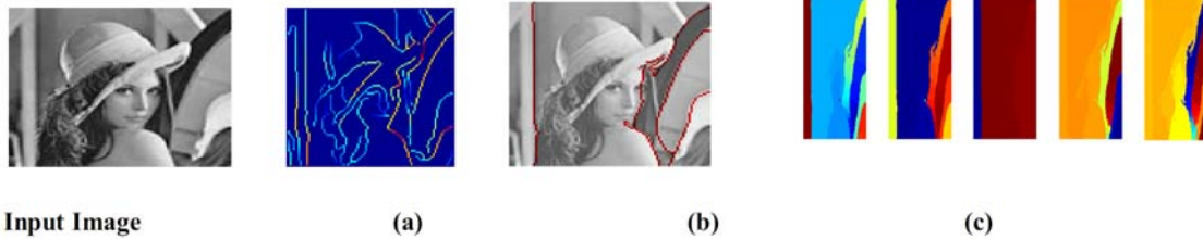
Fig. Output images of 100*100 size (a) Edge computed, (b) Segmented image, (c) Pseudo color segmentation
