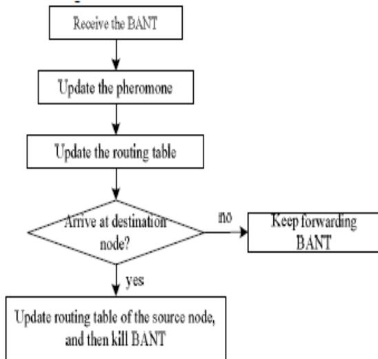
Fig. 5 The process of the BANT disposing
