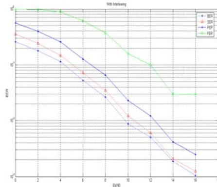
Fig.(10) Plot of BER,FER,SER and PEP v/s  $E_b/N_0$  (Logarithmic value) with interleaving.
