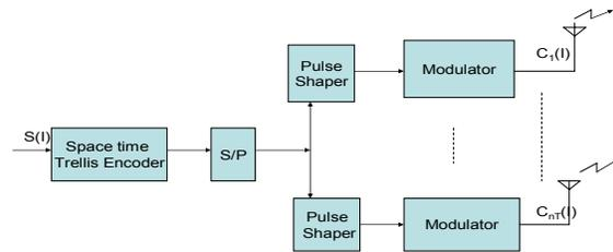
Fig.(3) A block diagram of a STTC based system.
