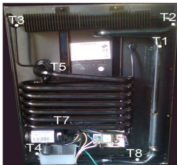
Figure 1: Placement of Thermocouples
