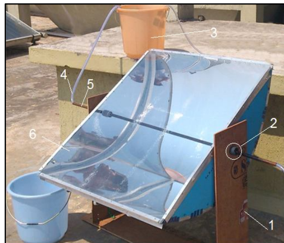
Figure 10: Thermal Collector with Thermosiphon Circulation
