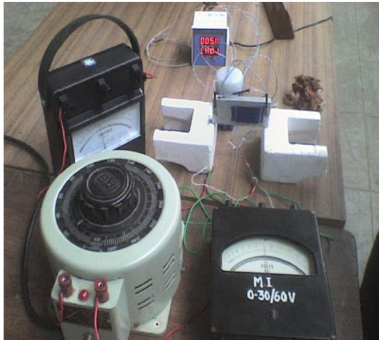
Fig. 2 Experimental setup with heat sink kept in the open air
