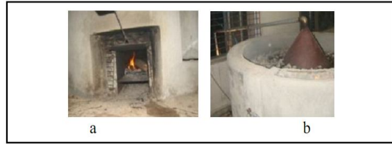
Figure 5. New furnace in operation: (a) Flaps covering entry point of combustion chamber, ash formed on combustion of firewood pulled out from underneath (b) rock insulation and piping from furnace fed to condenser for bamboo vinegar production.
