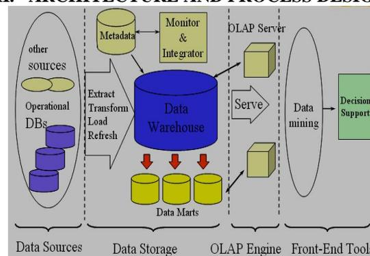
Figure: OLAP with data warehousing architecture
