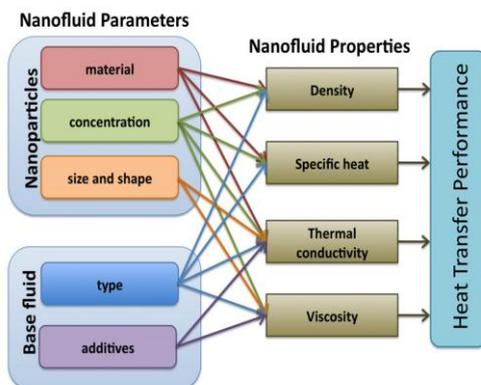
Fig: 4 Complexity and multi-variability of nanoparticle suspensions
