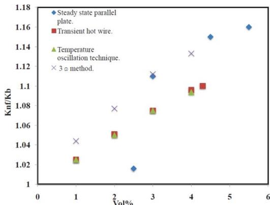
**3. Effect of volume fraction of nanoparticles on thermal conductivity of Al2O3-based nanofluids**
