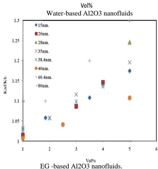
**5. Effect of base fluids on thermal conductivity of Al2O3- based nanofluids**
