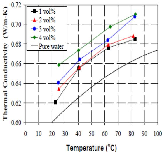
**2. Thermal conductivity of Al2O3 nanofluids measured by different techniques**
