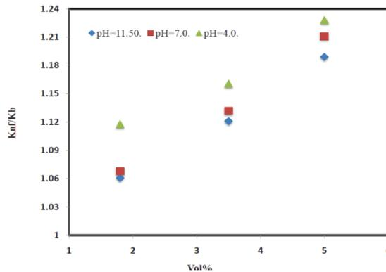
**8. Effect of surface active agents on thermal conductivity of water-based Al2O3 nanofluids**
