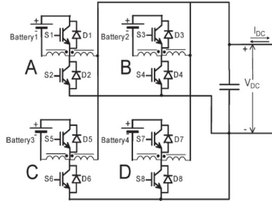
Figure 2: Four-phase bidirectional fly-back converter
