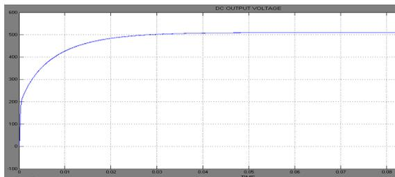
Figure 7: Output Voltage of the fly-back converter
