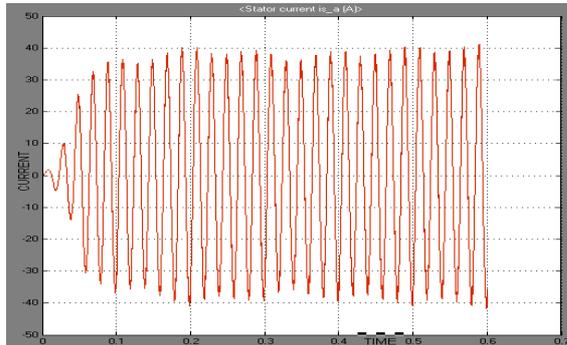
Figure 14: Stator Current of the Induction Motor Drive
