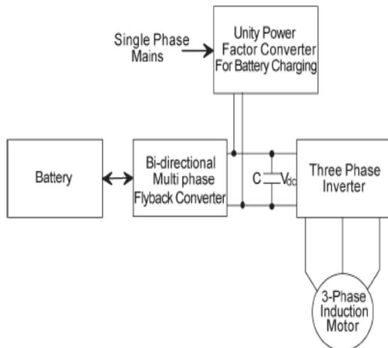
Figure 1. Block diagram of the proposed power schematic
