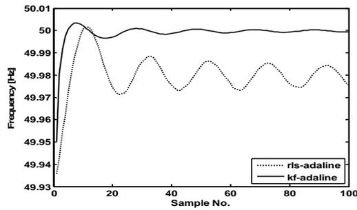
Fig. 3 Estimation of frequency at SNR 40 dB
