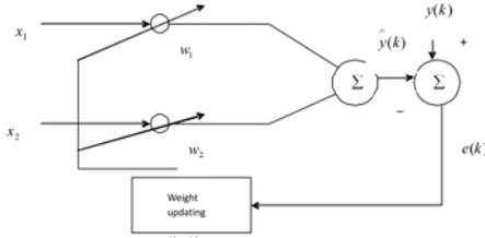
Fig. 1 shows the block diagrammatic representation of hybrid Adaline estimation scheme. First input signal is fed to Adaline structure. Output of Adaline is compared with the desired/reference output and the error so obtained is minimized by updating the weights of the Adaline using RLS/KF algorithm.
