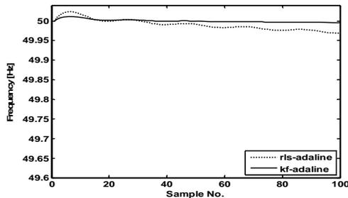
Fig. 6 Estimation of Frequency in presence of harmonics
