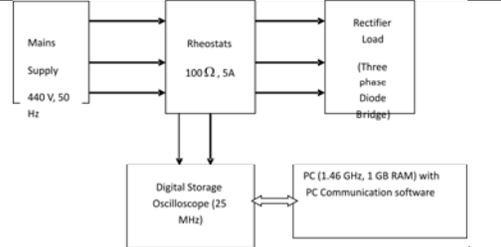
Fig.7 Experimental setup for online data generation
