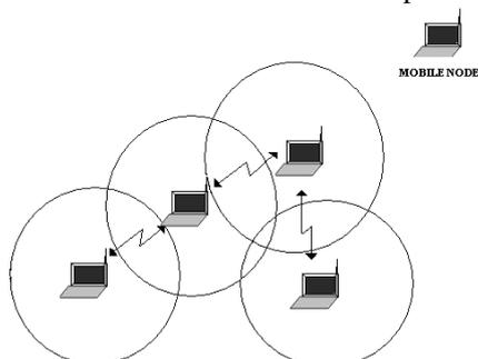
Figure 1: Ad Hoc Network System Architecture
