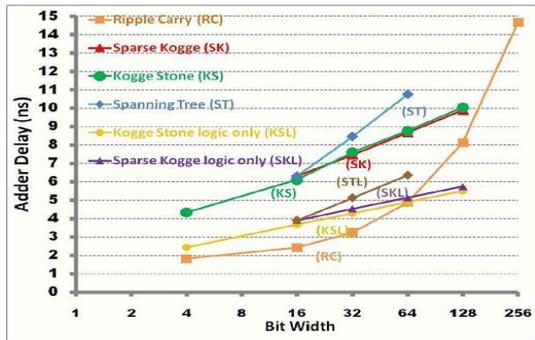
Fig. 6 . Simulation results for the adder designs
