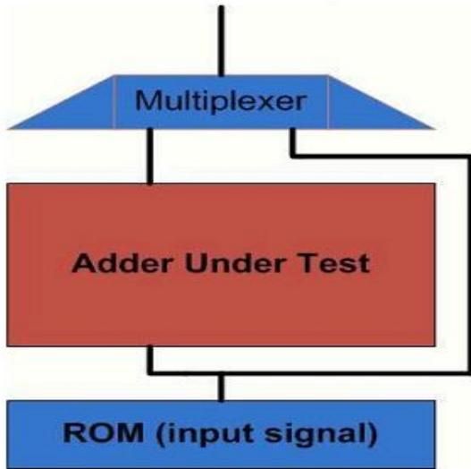
Fig. 3 . Circuit used to test the adders
