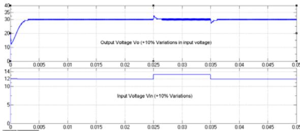
Fig-11 Output Voltage Waveform in Simple PID Controller (+10% Variations in Input Voltage)
