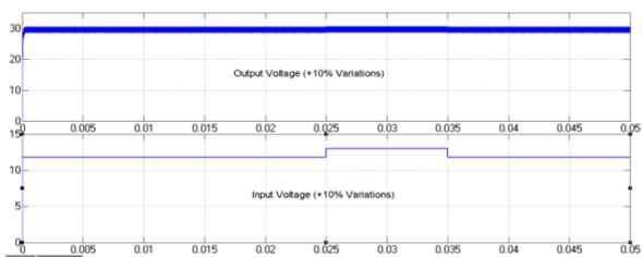
Fig-12 Output Voltage Waveform in FPGA Based Digital PID Controller ( $\pm$ 10% Variations in Input Voltage)
