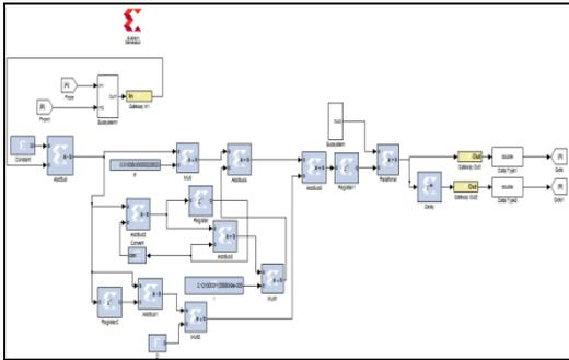
Fig-4 Sys Gen Implementation of PID Controller
