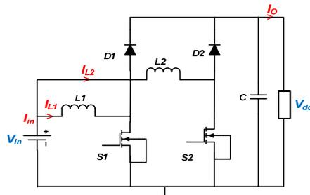
Fig.1 Two Phase Interleaved Boost Converter
