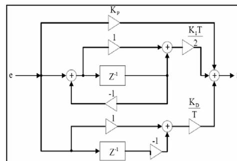
Fig-3 Direct Form Structure of Digital PID Controller
