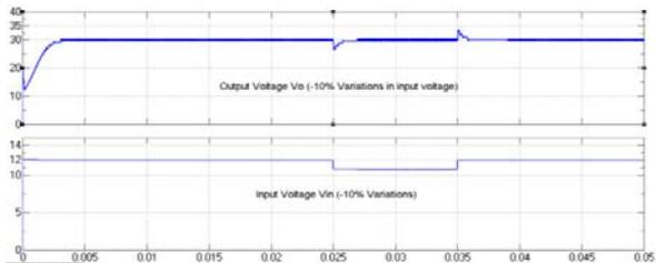
Fig-11a Output Voltage Waveform in Simple PID Controller (10% Variations in Input Voltage)
