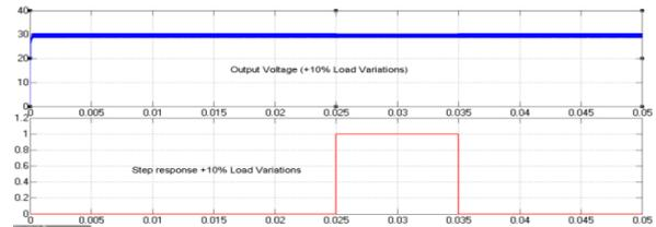
Fig-14 Output Voltage Waveform in FPGA Based Digital PID Controller (+10% Variations in Load)
