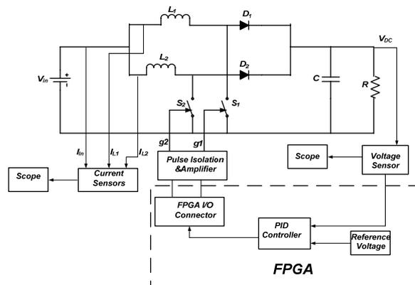
Fig-7 Block Diagram of Control and Power Scheme
