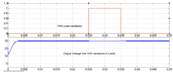
Fig-13a Output Voltage Waveform in Simple PID Controller (-10% Variations in Load)
