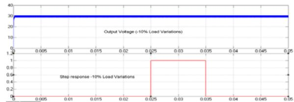
Fig-14a Output Voltage Waveform in FPGA Based Digital PID Controller (+10% Variations in Load)
