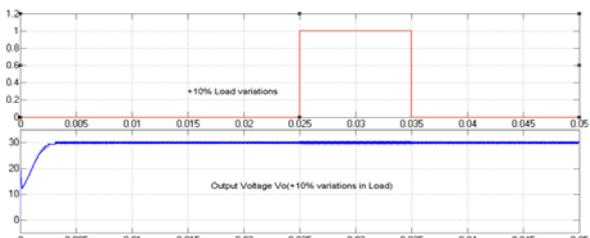
Fig-13 Output Voltage Waveform in Simple PID Controller (+10% Variations in Load)
