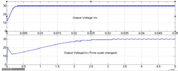
Fig-9 Output Voltage Waveforms in Simple PID Control (Stabilizing at 3.1 ms)
