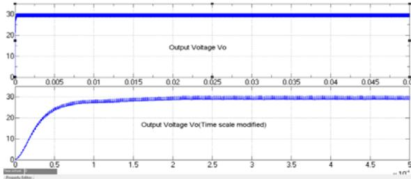
Fig-10 Output Voltage Waveforms in FPGA Based Digital PID Control (Stabilizing at 250  $\mu$ s)
