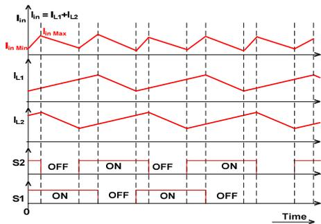
Fig-1a Typical Waveforms of Inductor currents (d > 0.5)
