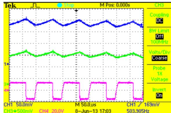
Fig-16 Inductor current, Source Current and Inductor Voltage Waveform
