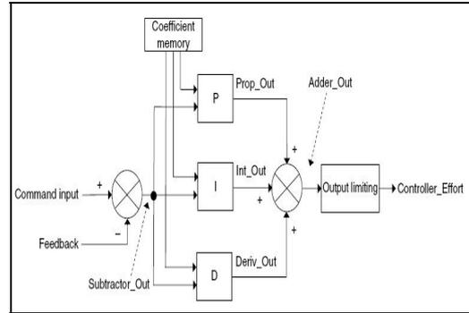
Fig-2 Digital PID Controller
