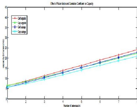
Fig. 2.12: MIMOCapacity vs. N with L=10,  $\rho=0.5$
