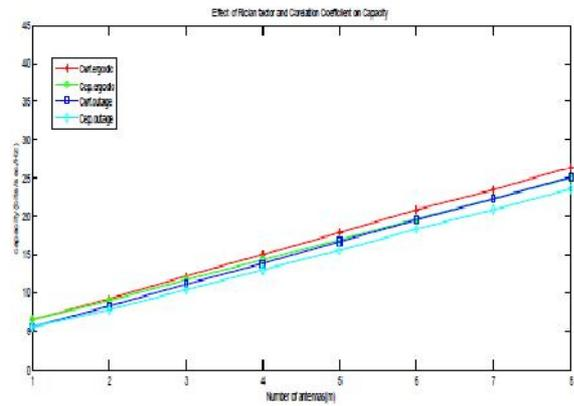
Fig. 2.11: MIMOCapacity vs. N with L=10,  $\rho=0.3$
