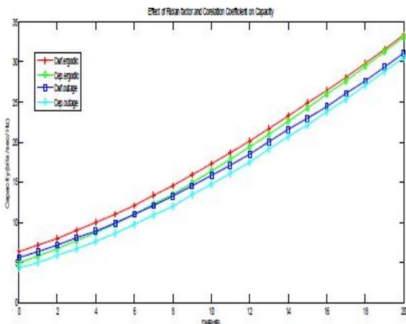
Fig: 1.1: MIMOCapacity vs. SNR, with L=0,  $\rho=0$
