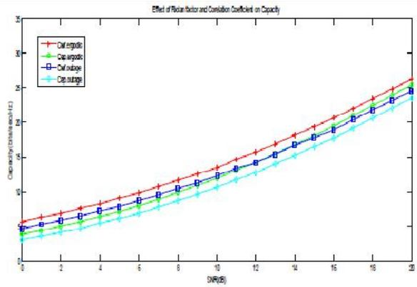
Fig: 1.2: MIMOCapacity vs. SNR, with L=0,  $\rho=0.7$
