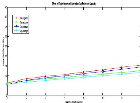
Fig. 2.13: MIMOCapacity vs. N with L=10,  $\rho=0.9$
