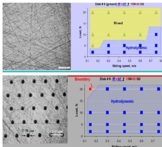
Fig.7 : Comparison of lubrication performance of un-textured (top) and laser-textured (bottom) surfaces.
