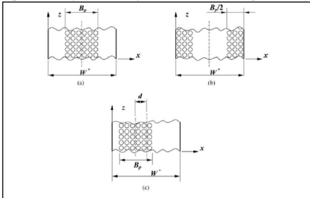
Fig. 4 : Different locations of the textured zone: (a) symmetrically in the center, (b) symmetrically at both ends, and (c) arbitrarily at a distance from the ring center.
