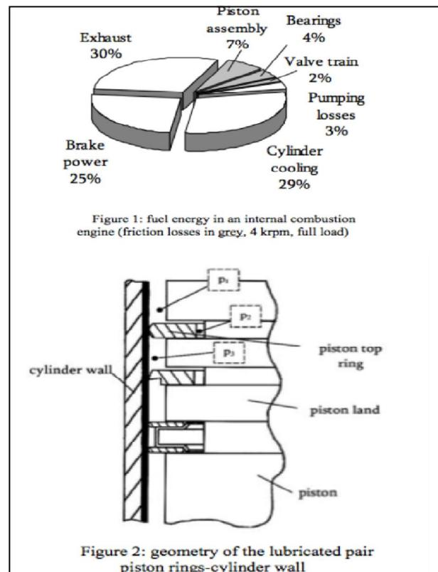
Proper lubrication and surface texture are key issues in reducing friction in a piston/cylinder system and, hence, have received a great deal of attention in the relevant literature. Surface texturing as a means for enhancing tribological properties of mechanical components has been well known for many years. Surface texturing in general and laser surface texturing (LST) in particular has emerged in recent years as a potential new technology to reduce friction in mechanical components.
