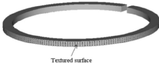
Fig. 3 : Laser Textured Piston Rings
