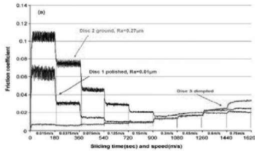
Fig. 8: Adding dimples delayed the onset of asperity contact in this test, from Kovalchenko, et. al. [12]
