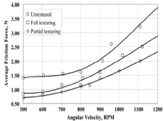
Fig. 5 : Time-averaged friction force vs. crank angular velocity for external normal pressure 0.1 MPa.
