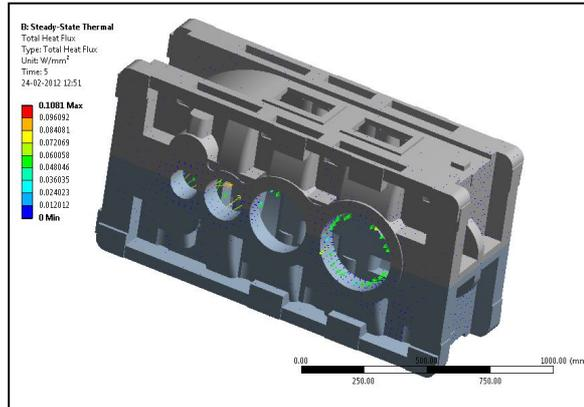
**Fig. 7 : Heat flux of gearbox casing**
