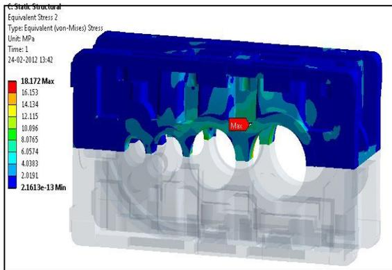
**Fig. 8 : Von-mises stresses on upper gearbox casing**
