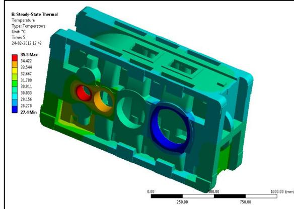
**Fig. 6 : Temperatures effect on gearbox casing,**
