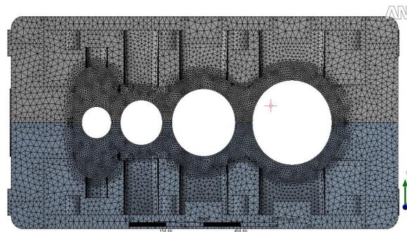
Fig. 2 : FEA model of gearbox casing
