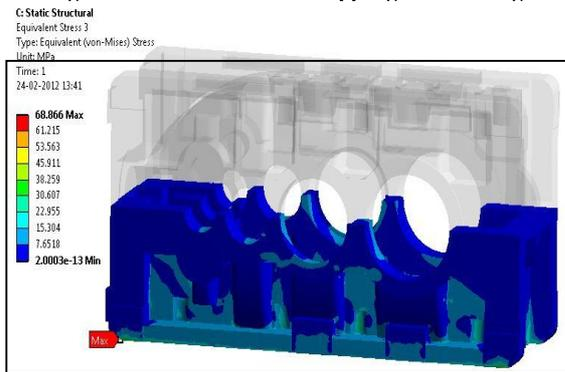
**Fig. 9 : Von-mises stresses on lower gearbox casing**
