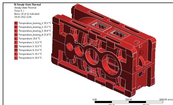
Fig. 3 : Thermal boundary condition of gearbox casing
