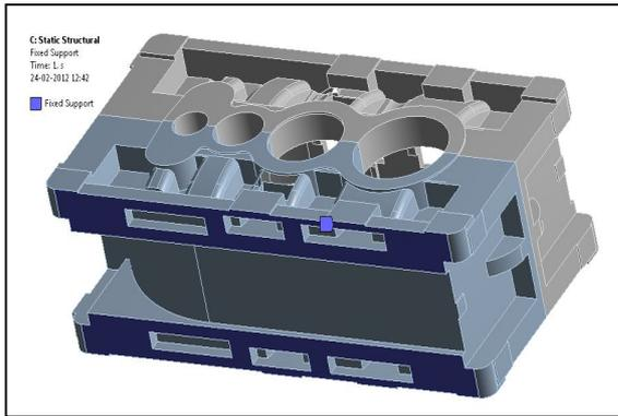
**Fig. 4 : Fixed support of bottom in gearbox casing**
