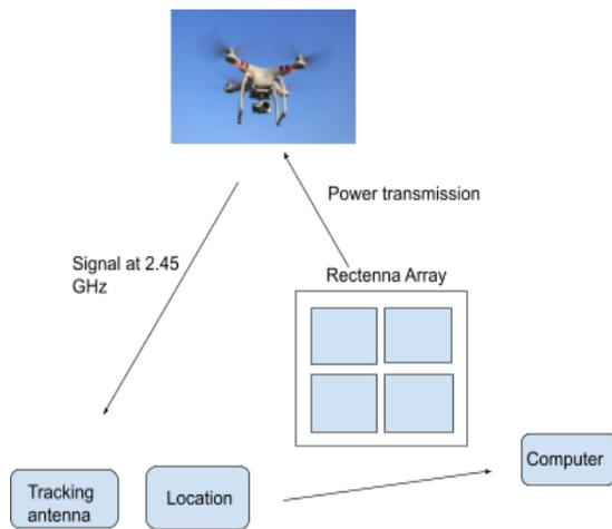
**Fig.3 Wireless power transmission in a Quadcopter**
