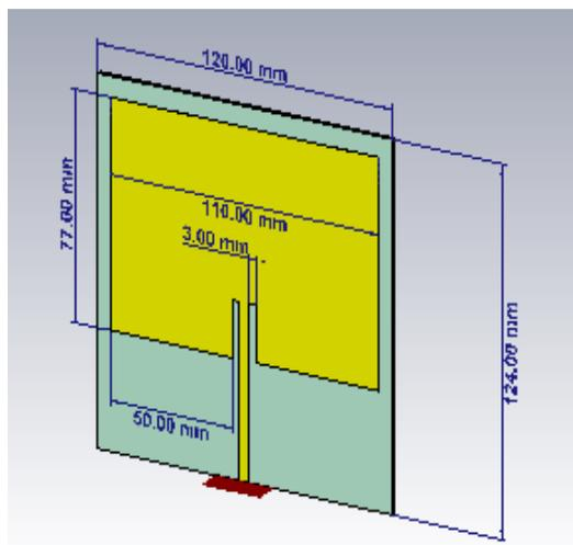
**Fig.5 Orthogonal view with dimensions**
