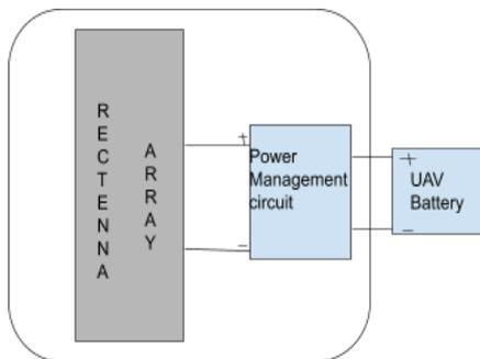
**Fig.8 Circuit Integration of Patch antenna and Rectifier**
