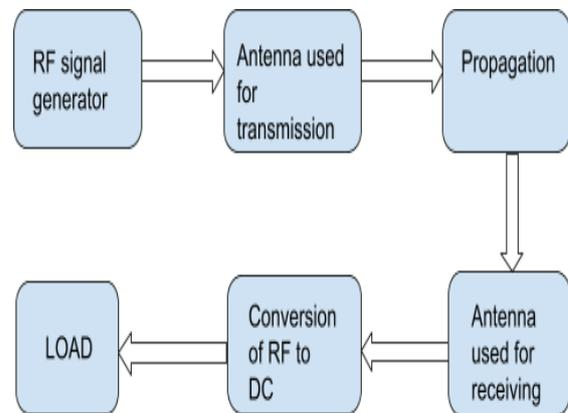
**Fig.2 Block diagram of wireless charging**
