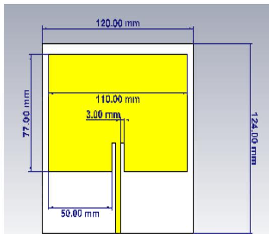
**Fig.4 Front view of patch antenna**
