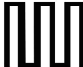
Fig.1 Meander Line Structure
