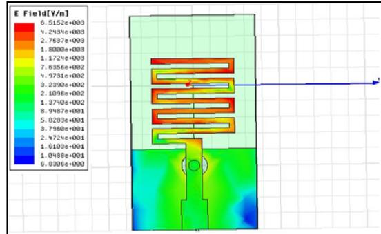
Fig.5 Surface current distribution on MLA at 2.5 GHz
