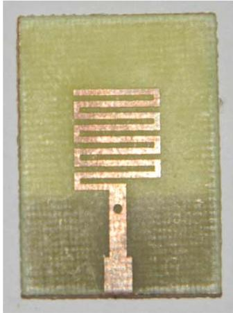
Fig.7 Photo of the fabricated antenna without connector
