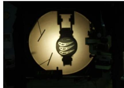
Fig. 5 : Inspection of cut-sections of turbine blade in optical profile projector
