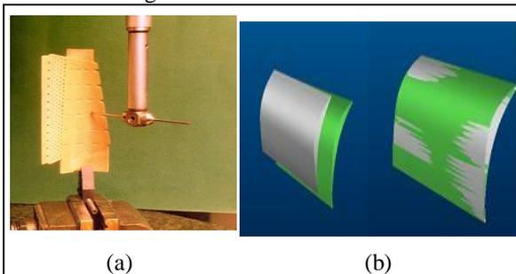
Fig. 3 (a) CMM inspection of a fired core and (b) CAD based best-fit analysis
