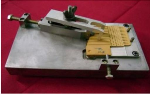
Fig. 15 : Core finishing fixture
