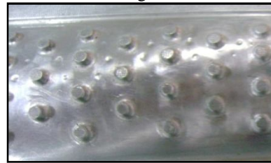
Fig. 7 : Surface degradation in ceramic core die made in aluminum
