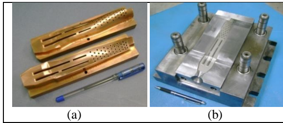
Fig. 8 : EDM electrodes and ceramic core die
