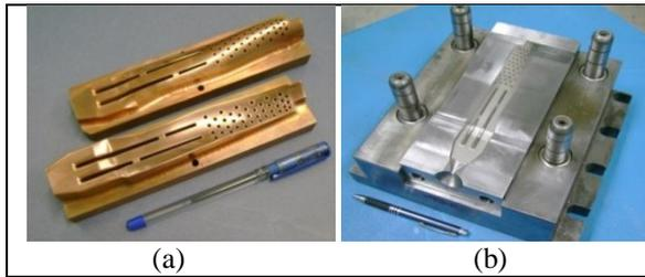
Fig. 8 : EDM electrodes and ceramic core die
