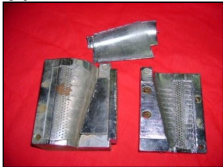
Fig. 6 : Soft tooling through rapid prototyping
