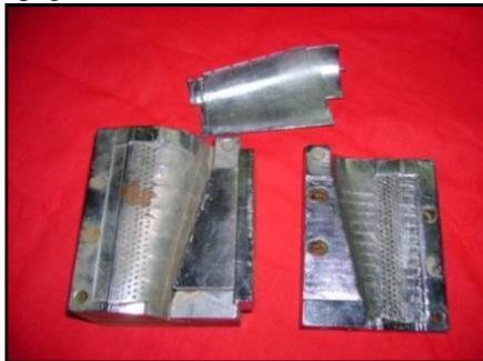
Fig. 6 : Soft tooling through rapid prototyping
