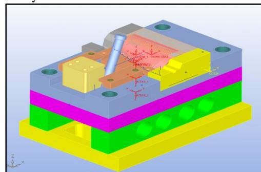
Fig. 11 : Design of mold base with finger cam
