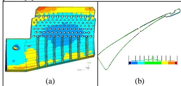
Fig. 4 : Deviation color mapping of a ceramic core using Laser CMM (a) entire surface and (b) sectional profile
