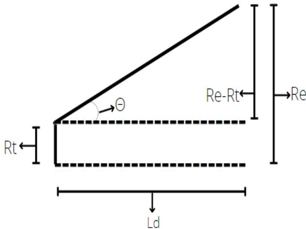
Figure 4. Divergent section of the Nozzle
