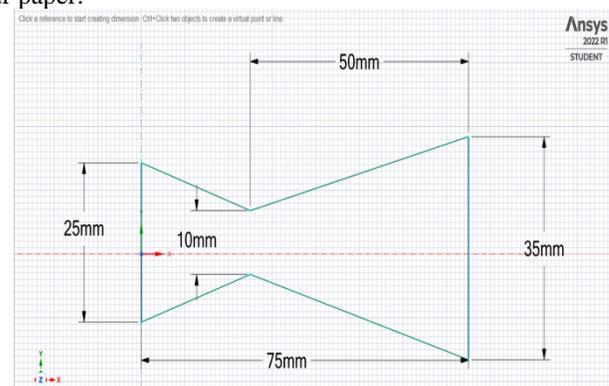
Figure 1. Schematic design of a standard C-D nozzle
