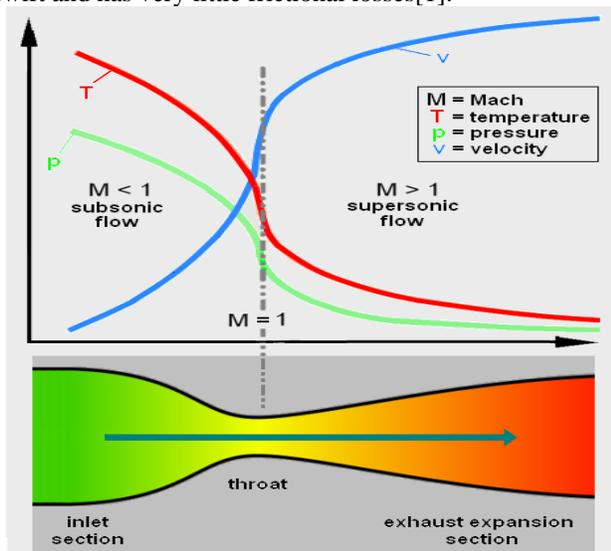
Figure 3. Graphic represents gas flow via a de Laval nozzle used to achieve supersonic velocity of rocket engine exhaust gases[3].
