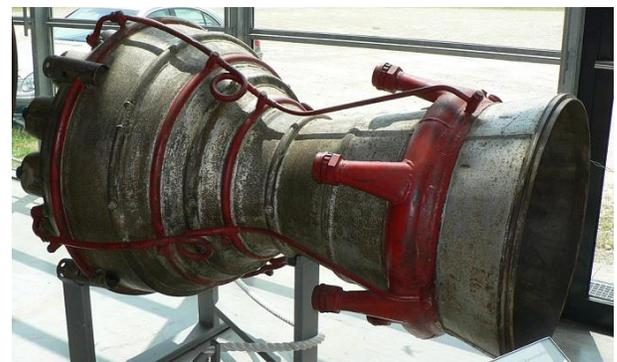
Figure 2. A real life C-D or (De Laval ) Nozzle [4]
