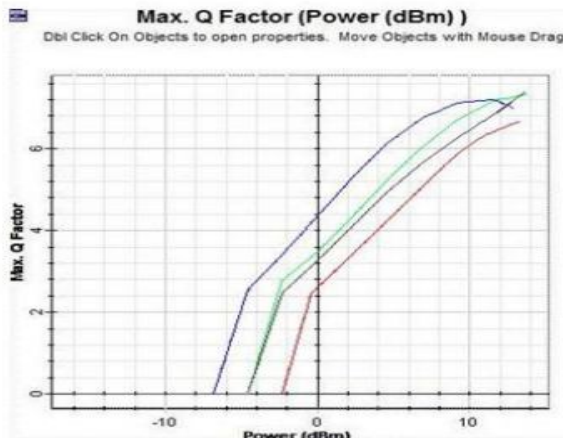
Figure 7: Q factor vs. Fixed received power for Post-compensation method Q=7.2
