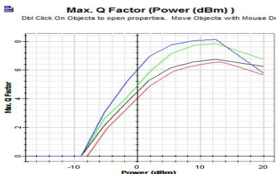
Figure 8: Q factor vs. Fixed received power for Pre-compensation method Q=9.4
