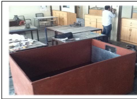
Fig. 7. Mild Steel Tank (6 feet * 4 feet * 3 feet)
