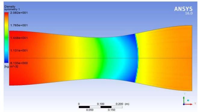
Figure:13 Density variation in shockwave
