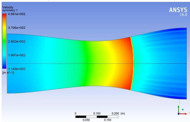
Figure:11 Velocity variation during shockwave
