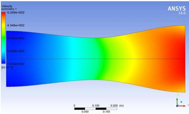
Figure:7 Velocity contour and graph (m/s)
