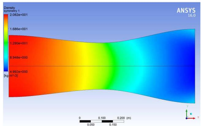
Figure:9 Density contour and graph ( $\text{kg/m}^3$ )
