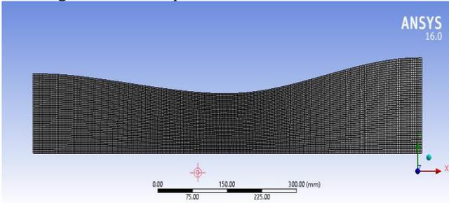
Figure:6 Meshed model of nozzle
