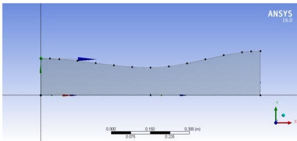
Figure:4 CAD model of nozzle
