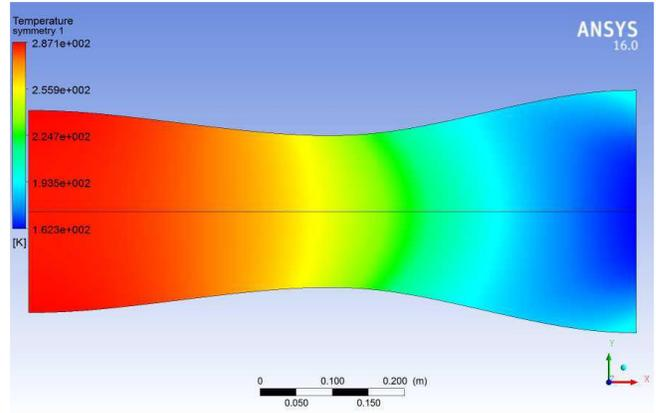
Figure:8 Temperature contour and graph (K)
