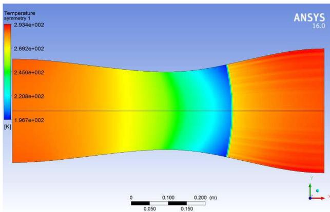
Figure:12 Temperature variation in shockwave
