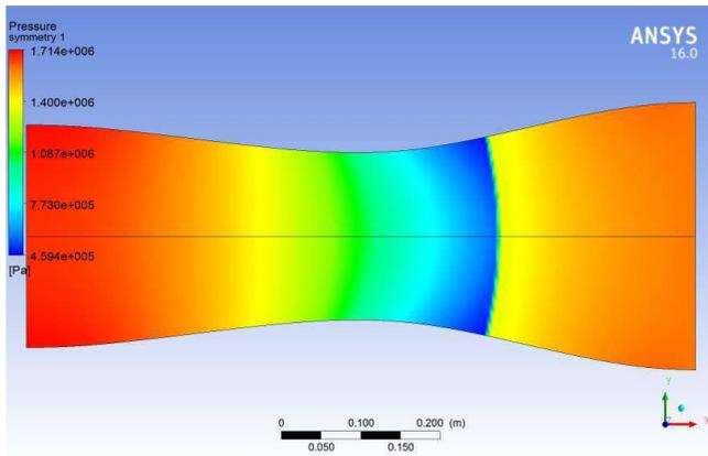
Figure:10 Pressure variation in shockwave
