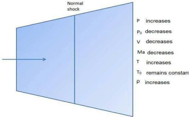
Figure:3 Variation of parameters in shockwave
