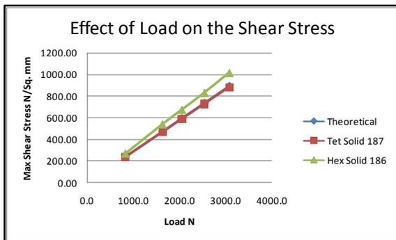
Figure 5-Load Vs Shear Stress Effect on spring
