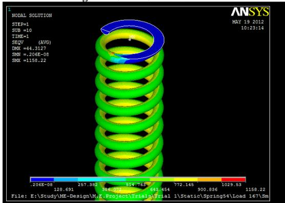
Figure 5-Eq. Von Mises Stress Counter
