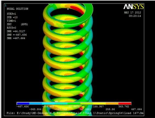
Figure 4-Shear Stress Counter
