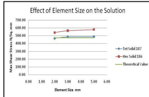
Figure 3- Comparison of Different Meshing Types
