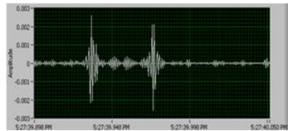
Fig. 12. Detection and localization of swell using WPT
