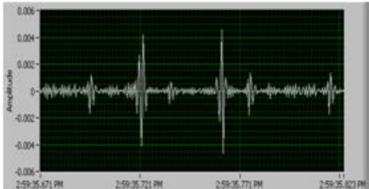
Fig.15. Detection and localization of sag by using WPT. The signal of voltage sag is simulated in LabVIEW® programming as shown in Fig. 14. The sampling frequency and supply frequency are 3.2 KHz and 50 Hz respectively. It is assumed that the lifting wavelet of Daubechies (db4) is decomposed to level 4. The coefficients of details at level 4 are shown in Fig. 15. A spike is seen at the starting and end point of the sag in WPT from time 5:59:35:721 to 5:30:00:768, from which, we can obtain the beginning time and the ending time of voltage sag accurately.[11]
