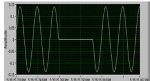
Fig. 8. Voltage interrupt signal shown in the front panel of LabVIEW®.
