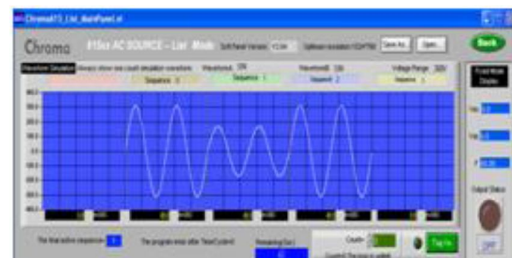
Fig 13. Waveform generation in chroma programming with sag disturbances
