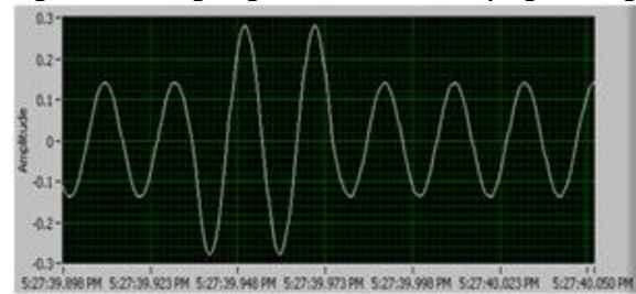
Fig.11. Swell voltage signal shown in the front panel of LabVIEW®
