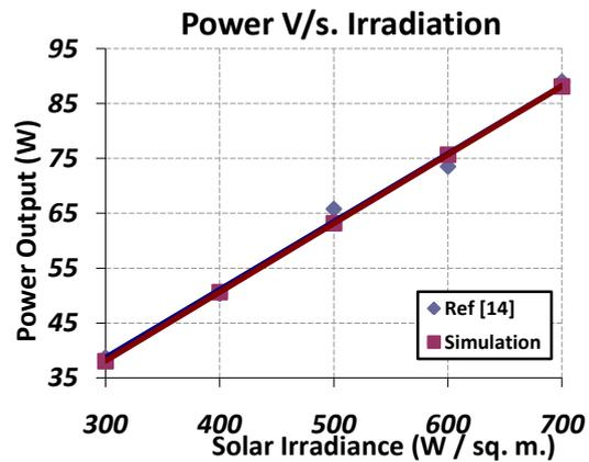
Figure 5. Relationship between the Electrical Power and Solar Irradiation at 25<sup>o</sup> C.
