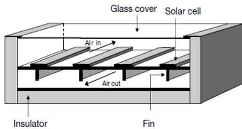
Figure 2. Finned Double-Pass Photovoltaic-Thermal Solar Air Heater [12]
