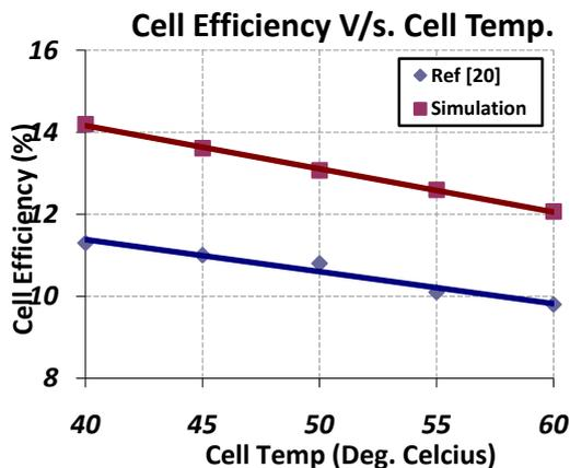
Figure 4. Relationship between the Electrical Efficiency and Cell Temperature at reference temperature of 25<sup>o</sup> C
