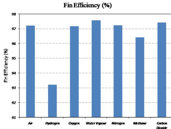
Figure 6. Comparison of Fin Efficiency for Various Gases.
