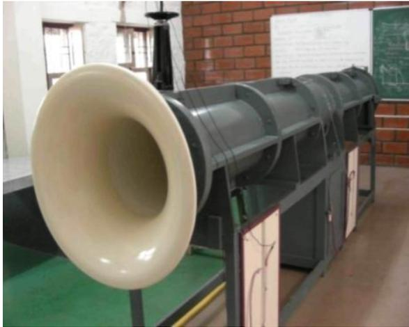
Fig: 2 Ducted Axial Fan Rig
