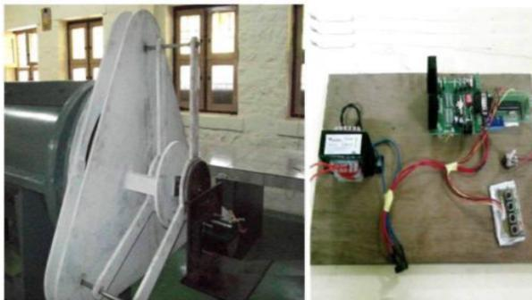
Fig.4. Variable frequency Drive for speed control
