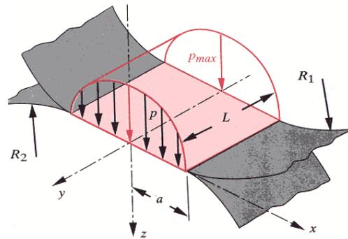
From Figure 3.4 the width of the contact zone is  $2a$ . If total contact force is  $F$  and contact pressure is  $p(x)$ , there is a formula [5], which shows the relationship between the
