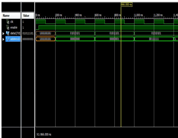
Fig 6 The data and state input (finite state machine s0 to s1 to s7)
