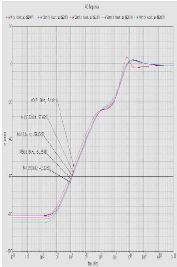
Fig.7. Measured PSRR at  $V_{IN} = 2.5V$ ,  $I_{load}$  from 0mA to 40mA.
