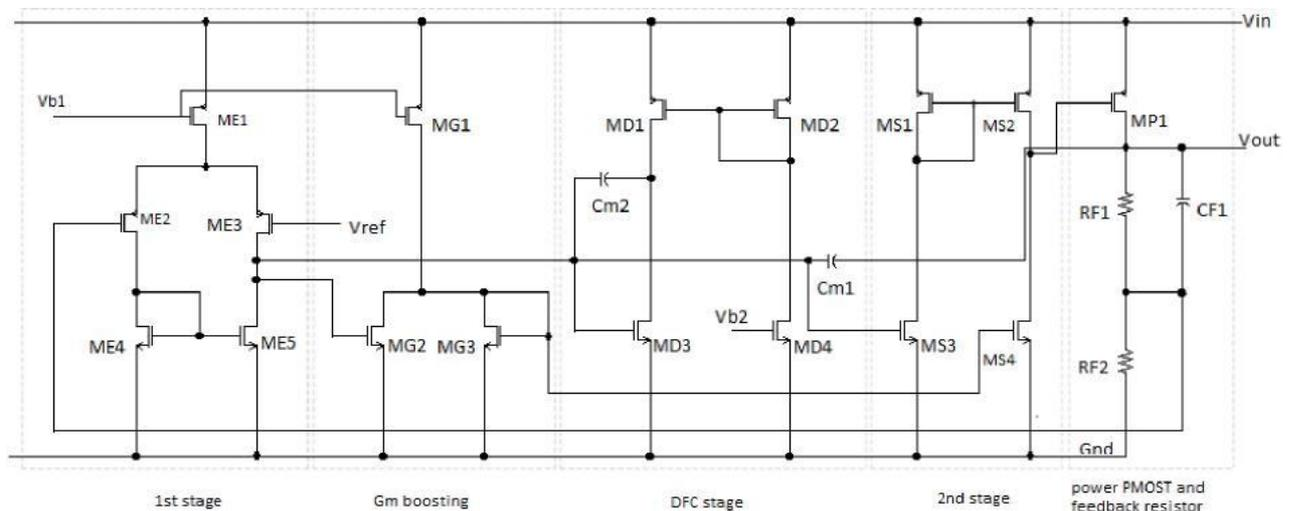
Fig. 3. Structure of the proposed LDO with capacitor-free feature.
