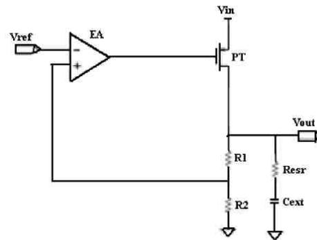
Fig 1 Conventional LDO voltage regulator
