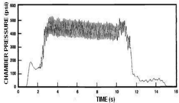
Fig. 3. Pressure oscillations as a result of combustion instabilities in a hybrid rocket motor[5]
