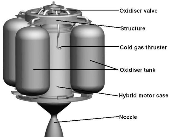
Fig. 4. A scheme of the Maneuvering and orbital Transfer Vehicle[3]
