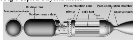
Fig. 1. Hybrid rocket motor scheme[2]
