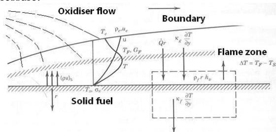
Fig. 2. A simplified model describing the hybrid motor combustion [2,3]
