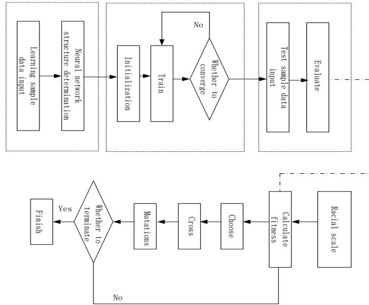
**Fig 1.** Operation flow of GA-BP neural network model
